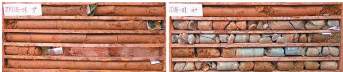
**Figure 4-13: Drill Cores Showing Relatively Good Recoveries of Mineralised Intervals
